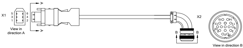
Figure 4-11 Absolute encoder motor wiring
